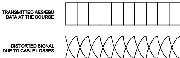
For balanced AES/EBU transmissions, 110Ω shielded, twisted pair cable is recommended and for unbalanced transmissions, 75Ω co-axial cable. As rectangular pulse digital signals are inherently rich in harmonics, they require a wide bandwidth for distortion-free transmission.
