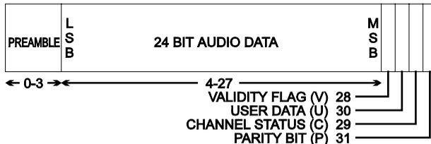
As illustrated in fig.1, a sub-frame consists of a preamble, 24 audio data bits, validity bit (V), user data bit (U), channel status bit (C) and sub-frame parity bit (P). Each stereo sample or frame comprises two sub-frames, A and B. Sub-frames A and B represent the left and right programme information of the stereo sample respectively.
